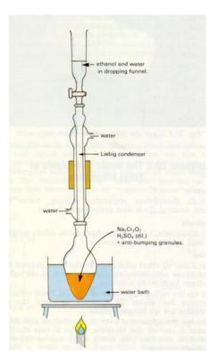
• Heat Ethanol with **acidified dichromate** in **reflux** apparatus for **30 mins.**
